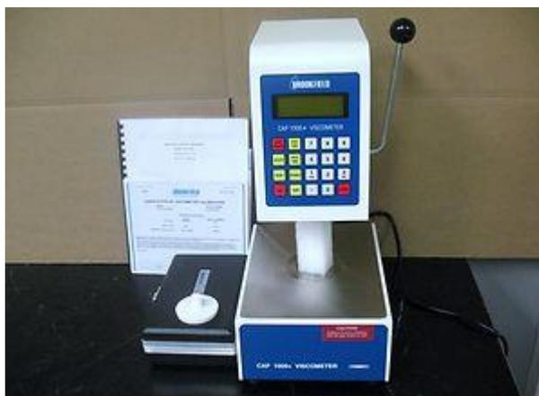
Gambar 2.5. *Viscometer Cone/ Plate*
