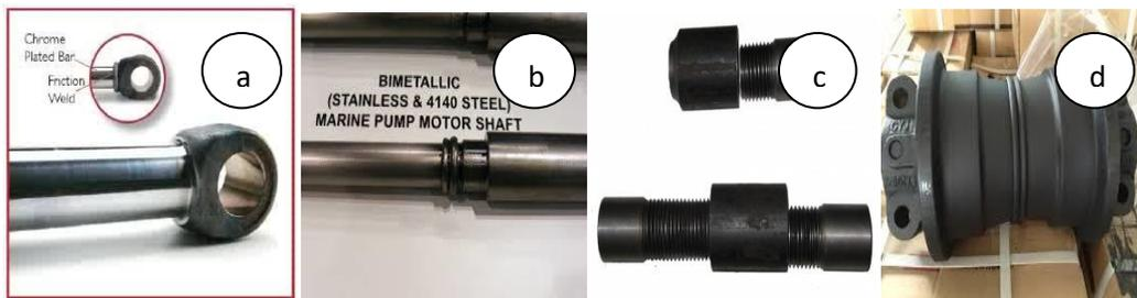
Gambar 2.4. Aplikasi pengelasan gesek Sumber :*Materials Azo*. 2015. *Friction Welding in the Manufacturing of OEM Chemical Processing Equipment - A Case Study by American Friction Welding*.
