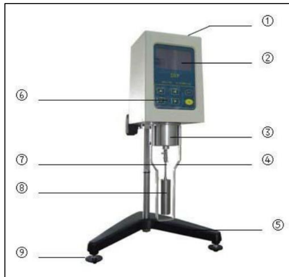
Gambar 3.21 Bagian-bagian vikometer NDJ 8S (Sumber : Manual book)
