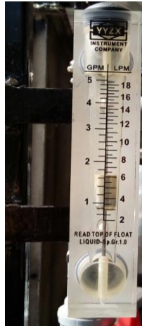
3. Flowmeter 5 GPM / 18 LPM
