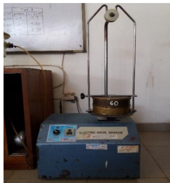
Gambar 3.7 Alat Penyaring ( Electric Sieve Shaker )
