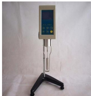
Gambar 3.7 Digital Rotary Viscometer
