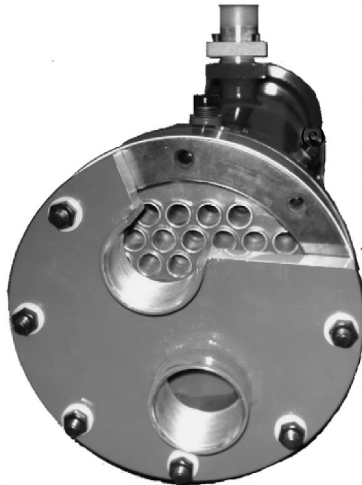
Gambar 2.8 Kondensor tipe Shell and Tube (Hundy, 2008)
