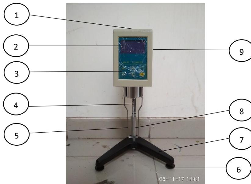
**Gambar 3.20.** Bagian-bagian Viskometer NDJ 8S
