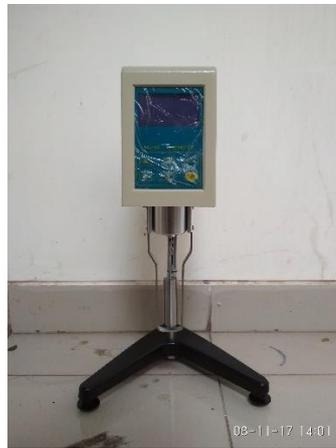
**Gambar 3.16.** Viskometer NDJ 8S
