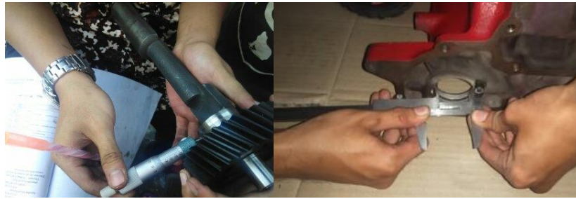
Gambar 4.6 Diameter bearing balancer dan Rumah balancer shaft
