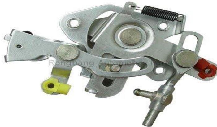
Gambar 2.15 *Door locking mechanisme* ( Anonim, tt )
