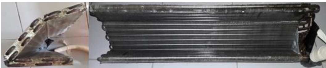
Gambar 3.5 Unit evaporator AC LG 3/4 PK
