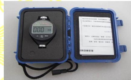
Gambar 4. *Shore Durometer*
