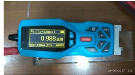
Gambar 3. Alat surface roughness tester.
