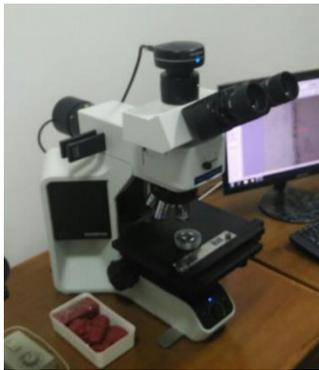
Gambar 6. *Metallurgical Microscope Olympus BX53M.*
