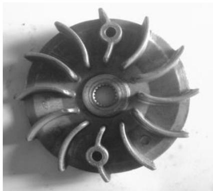
Gambar 2.11 *Pulley Tetap (Fixed Sheave)*
