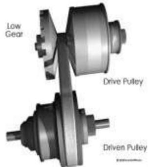
**Gambar 2.27** Mekanisme CVT (*Continue Variable Transmision*)
