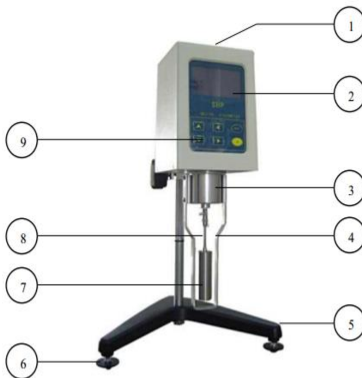
Gambar 3. 22 Rangkaian penyangga beserta viscometer NDJ 8S ( manual book viscometer NDJ 8S )
