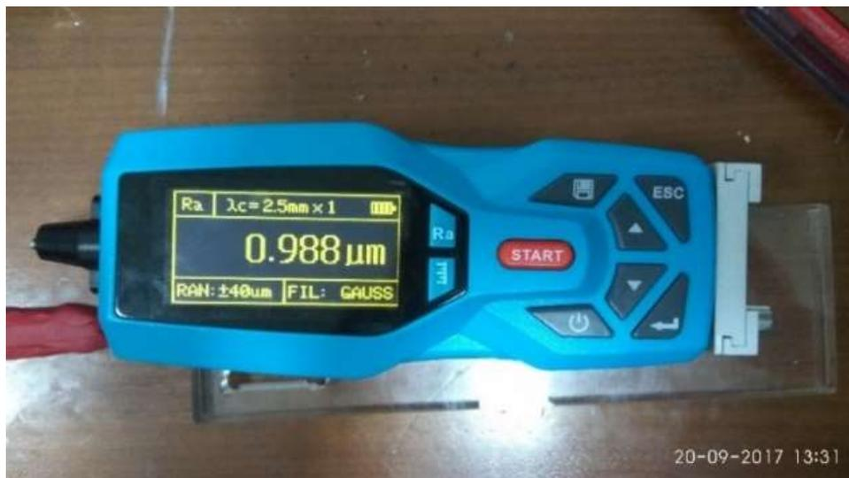
**Gambar 3.15.** Alat ukur kekasaran *Surface Roughness Measurement*.
