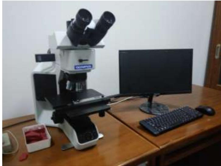
**Gambar 3.18.** Alat struktur lapisan *Metallurgical Microscope Olympus BX53M*
