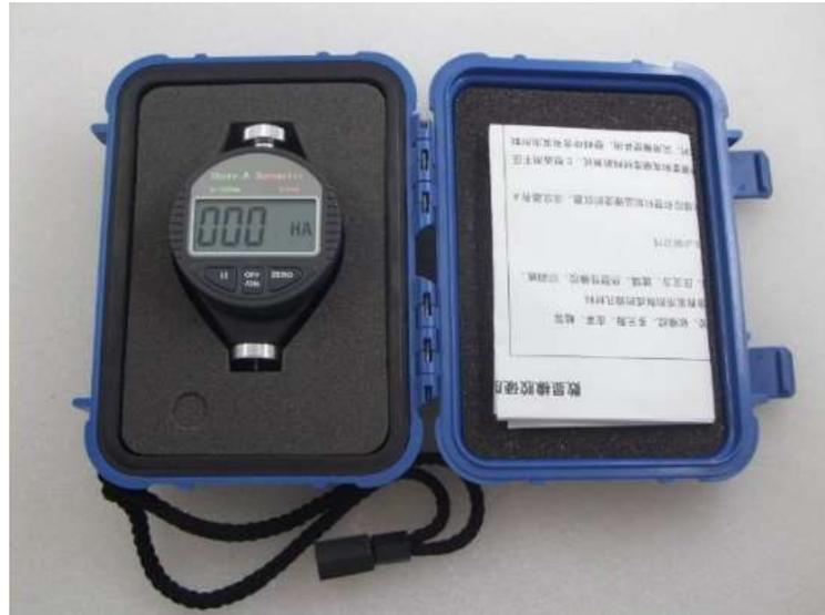
**Gambar 3.17.** Alat ukur kekerasan *Shore Durometers Hardness Tester*
