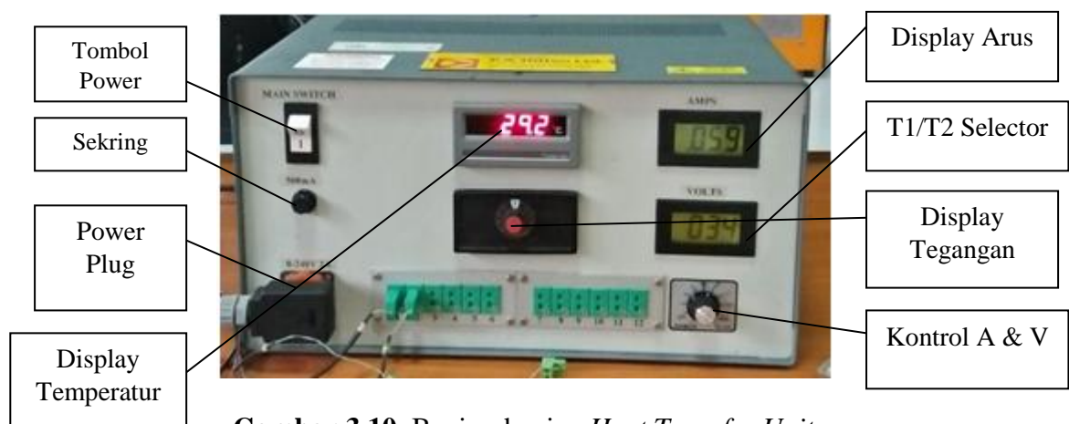
Gambar 3.10. Bagian-bagian Heat Transfer Unit
