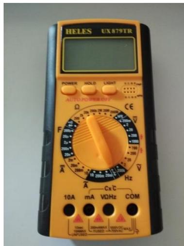
Gambar 3.21 Multimeter
