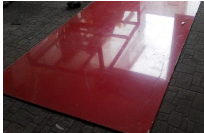
Gambar 4.27 Lembaran Plat ACP ( Aluminium Composite Panel )
