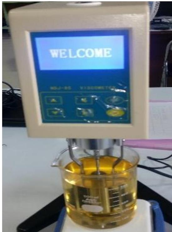
**Gambar 3.9.** Viskometer NDJ 8S
