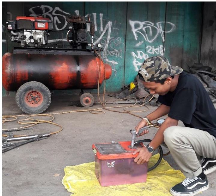
Gambar 3.14 Ilustrasi proses shot peening
