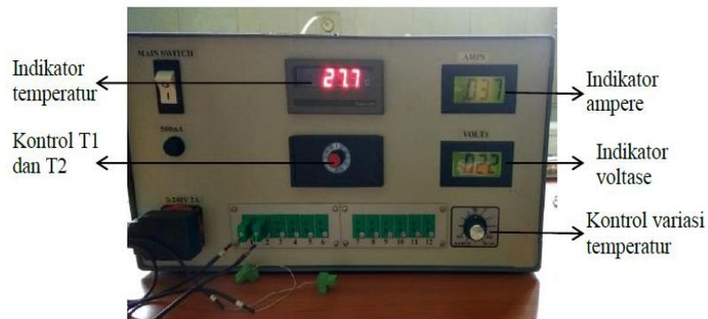
**Gambar 3.12.** Thermal Conductivity of Liquid And Gases Unit
