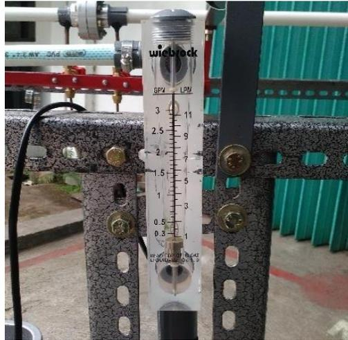
**Gambar 3. 5** Rotameter air
