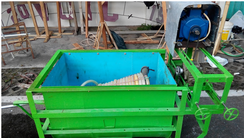
Gambar 3.1. Sling pump skala laboratorium
