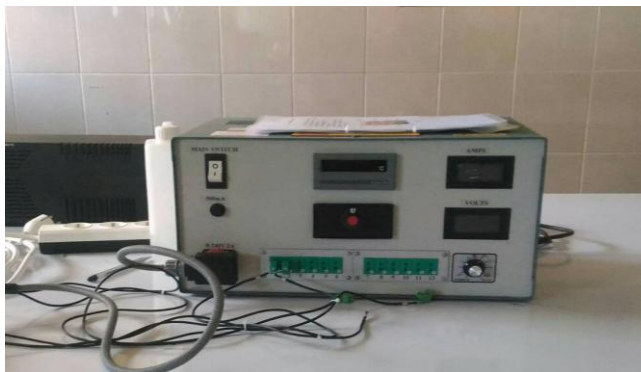
Gambar 3.5. Thermal conductivity of liquid and gases unit
