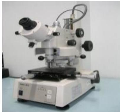
Gambar 3.5 Alat uji kekerasan micro Vickers
