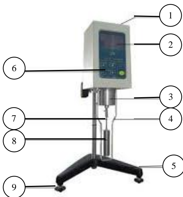
Gambar 3.14. Bagian–bagian viskometer NDJ 8S
