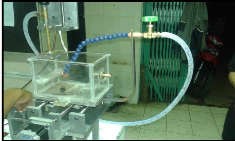
Gambar 3.19. Arah aliran (*flushing*) (Firdaus, 2015 dan Sulistiyo, 2016)
