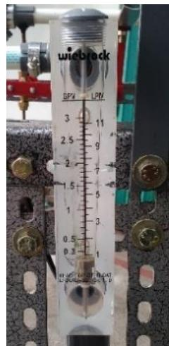
**Gambar 3. 5 Rotameter air**
