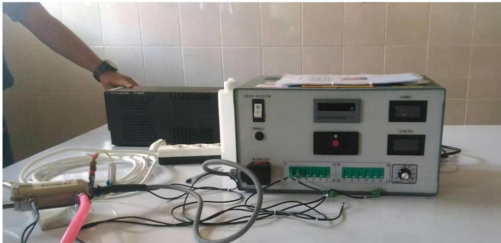
**Gambar 3.4** *Thermal Conductivity of Liquid And Gases Unit*
