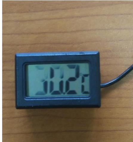
**Gambar 3.15** Termometer digital
