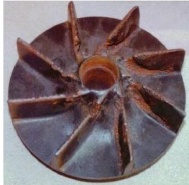
Gambar 2.8. Kerusakan Impeler Akibat Kavitasi (sumber : https://www.slideshare.net )
