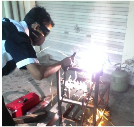
Gambar. 4.3. Pengelasan Braket Filter Solar
