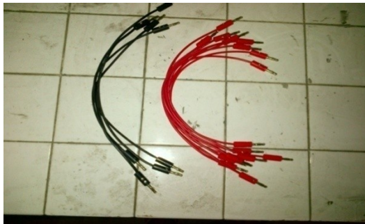
Gambar 4.7. Male Jack banana ukuran 30 cm.
