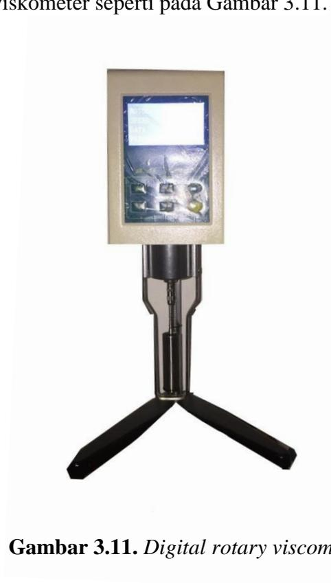
**Gambar 3.11.** *Digital rotary viscometer*
