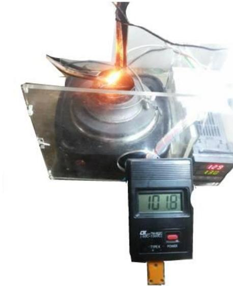
**Gambar 3.12.** Mesin *flash point*
