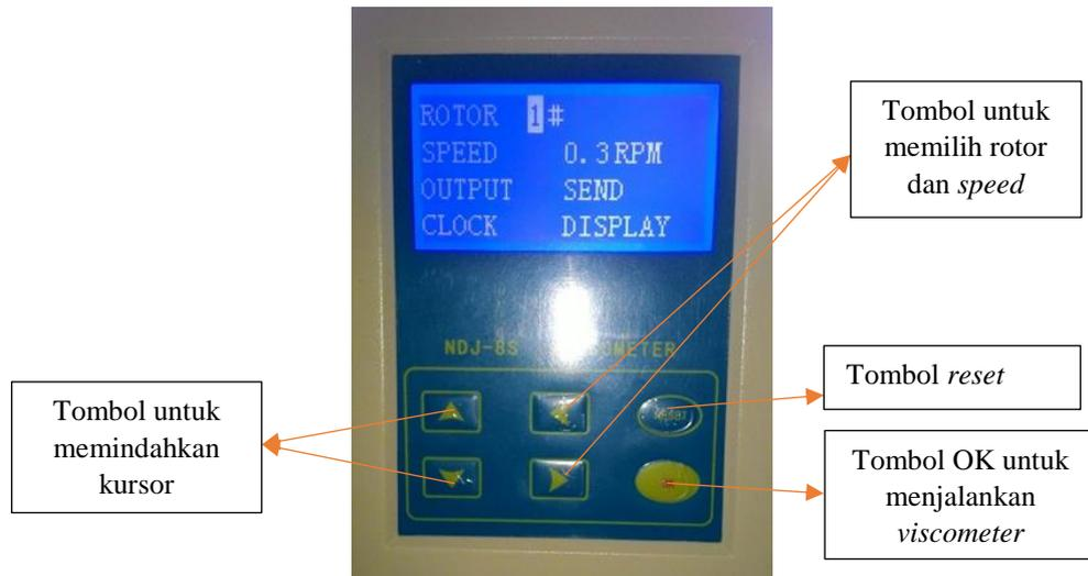
**Gambar 3.18.** Viskometer
