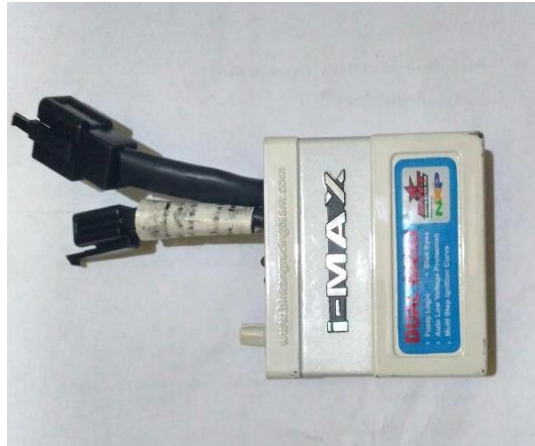
Gambar 3.4 CDI Racing BRT I-Max
