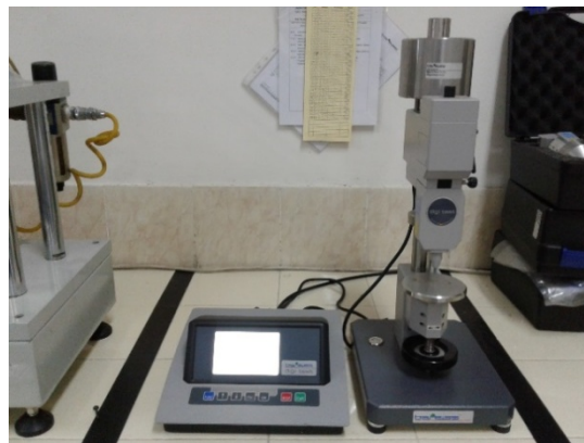
Gambar 3.5 Alat uji kekerasan Shore D (BBKPP Yogyakarta, 2017)
