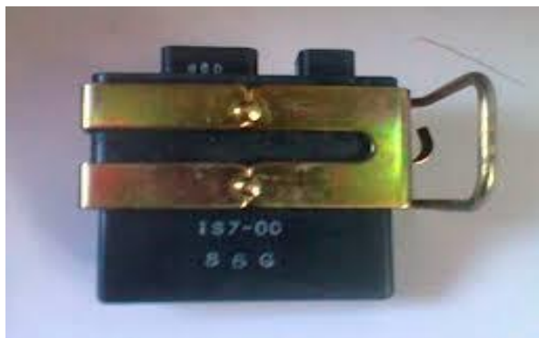
Gambar 2.5 CDI ( Capacitor Discharge Ignition )
