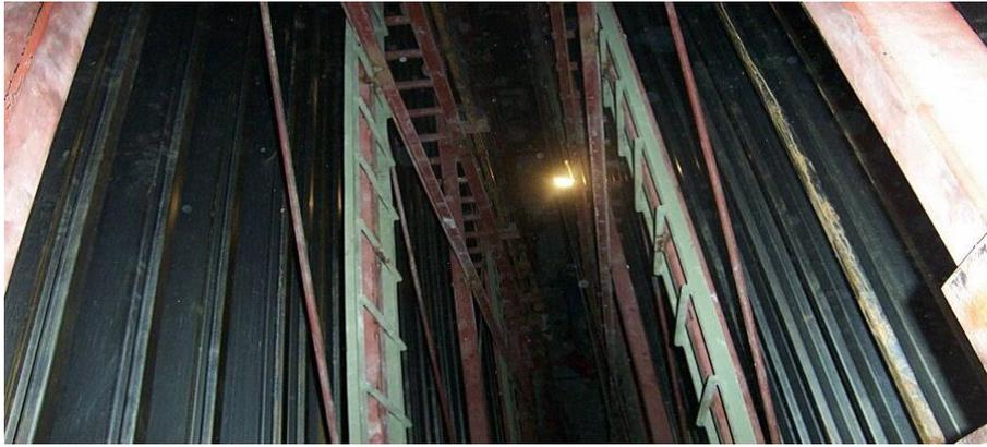
Gambar 2.5 Collecting Plate ESP
