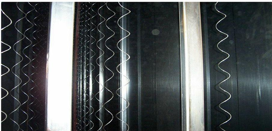
Gambar 2.6 Discharge wire ESP
