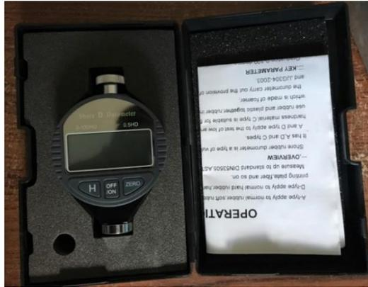
Gambar 3.3 Shore Hardness Tester, Type D
