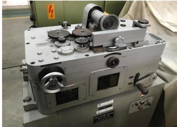
Gambar 3.5 *Ogoshi High Speed Universal Wear Testing Machine (Type OAT-U)*
