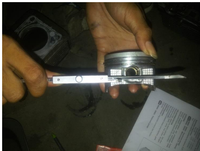
Gambar 3.11 Pengukuran Diameter Piston
