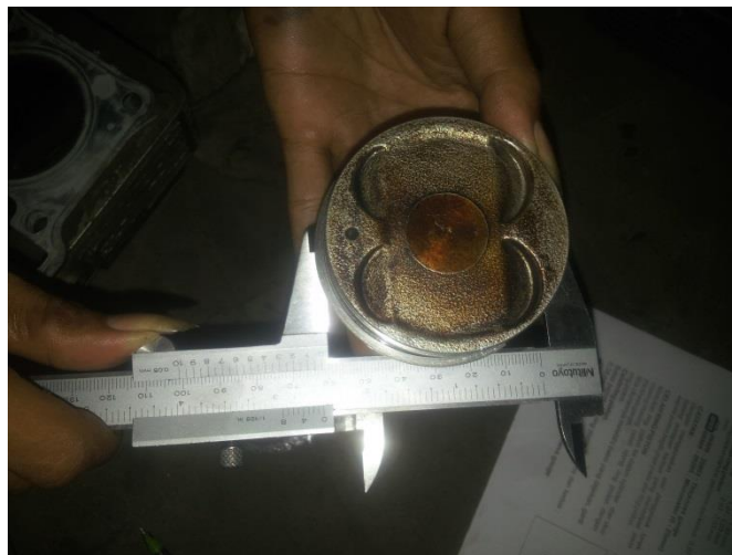
Gambar 3.10 Pengukuran Diameter Piston
