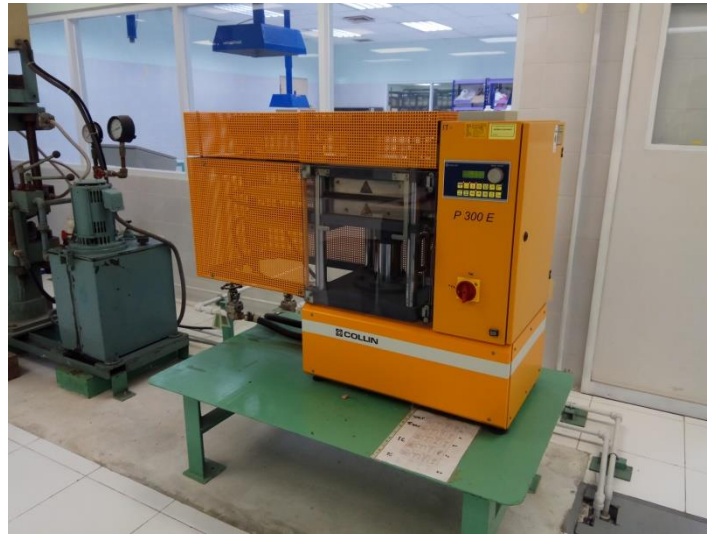
Gambar 3. 2 Alat Hot Press Molding Collin P300E
