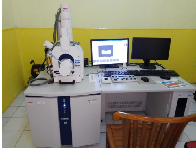
Gambar 3. 9 Scanning Electron Microscopy (SEM) Hitachi SU-3500
