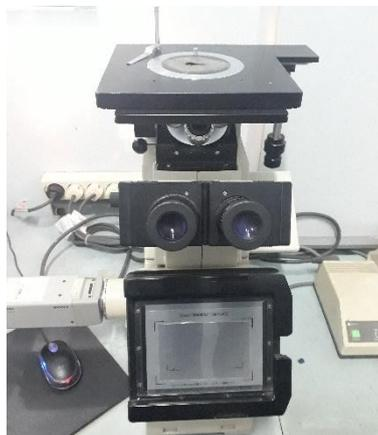
**Gambar 3.5.** *Metallurgical microscope inverted type*
