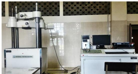
**Gambar 3.4.** Mesin uji tarik *Universal Testing Machine (UTM)*
