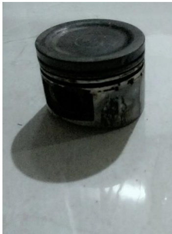
Gambar 3.4 Piston standard Yamaha Jupiter Z
