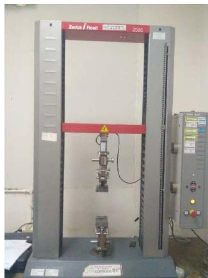
Gambar 3.3 *Universal Testing Machine* (UTM)
