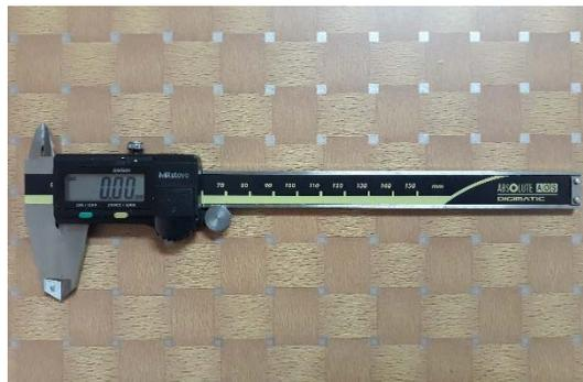
Gambar 3.7 Jangka Sorong Model Digital
