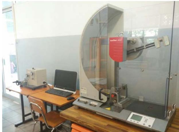
Gambar 3.4 Alat Uji Impak Model *Charpy*
