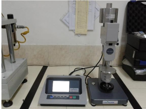
Gambar 3.5 Alat Uji Kekerasan Model Shore D
