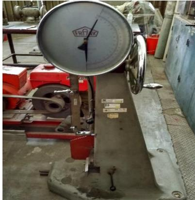
**Gambar 3.8** Alat Uji Impak *Charpy*
