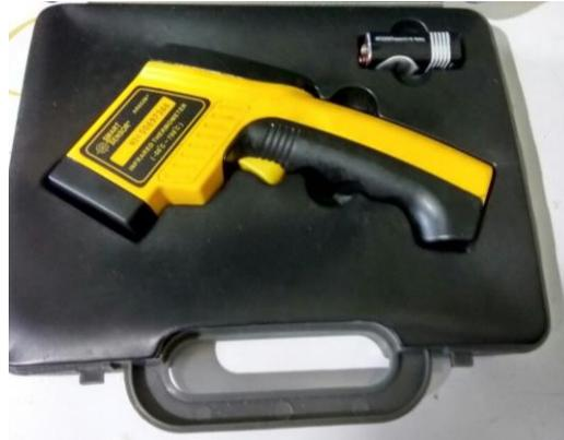
**Gambar 3.6** *Termo Infrared*
