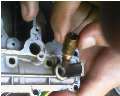
Gambar 3.12 Melepas pump plunger
