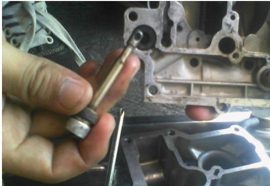
Gambar 3.12 Melepas pump plunger
