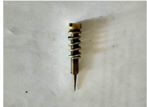
Gambar 4.11 Memeriksa idle adjusting screw
