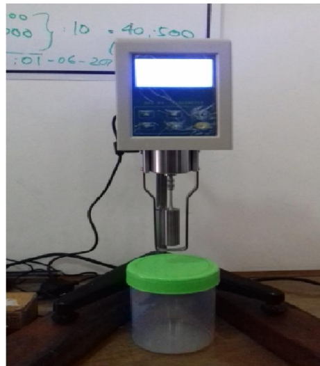
Gambar 3.13. Digital Rotary Viscometer
