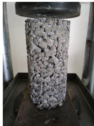
Gambar 4. Benda uji varian fly ash 60%
