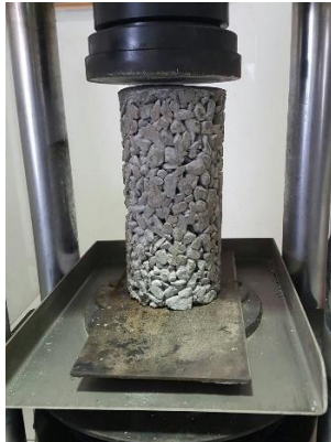
Gambar 1. Benda uji varian fly ash 0%
