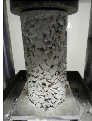
Gambar 2. Benda uji varian fly ash 20%
