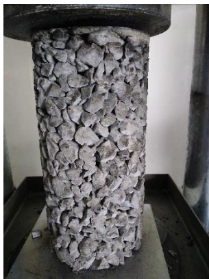
Gambar 3. Benda uji varian fly ash 40%
