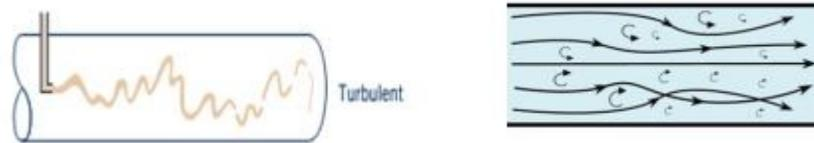
Gambar 2.9 Aliran Turbulen (Helmizar., 2010)
