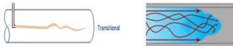
Gambar 2.10 Aliran Transisi (Helmizar., 2010)
