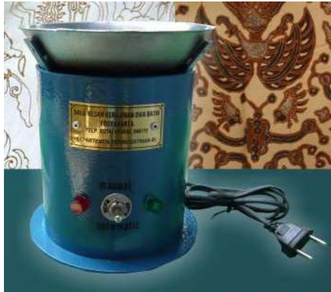
Fig. 3. Batik electric stove of 125 W, 220 volts.
